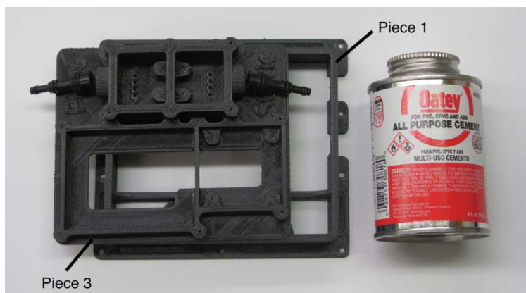
Parts before gluing (note cut Tee fitting)
